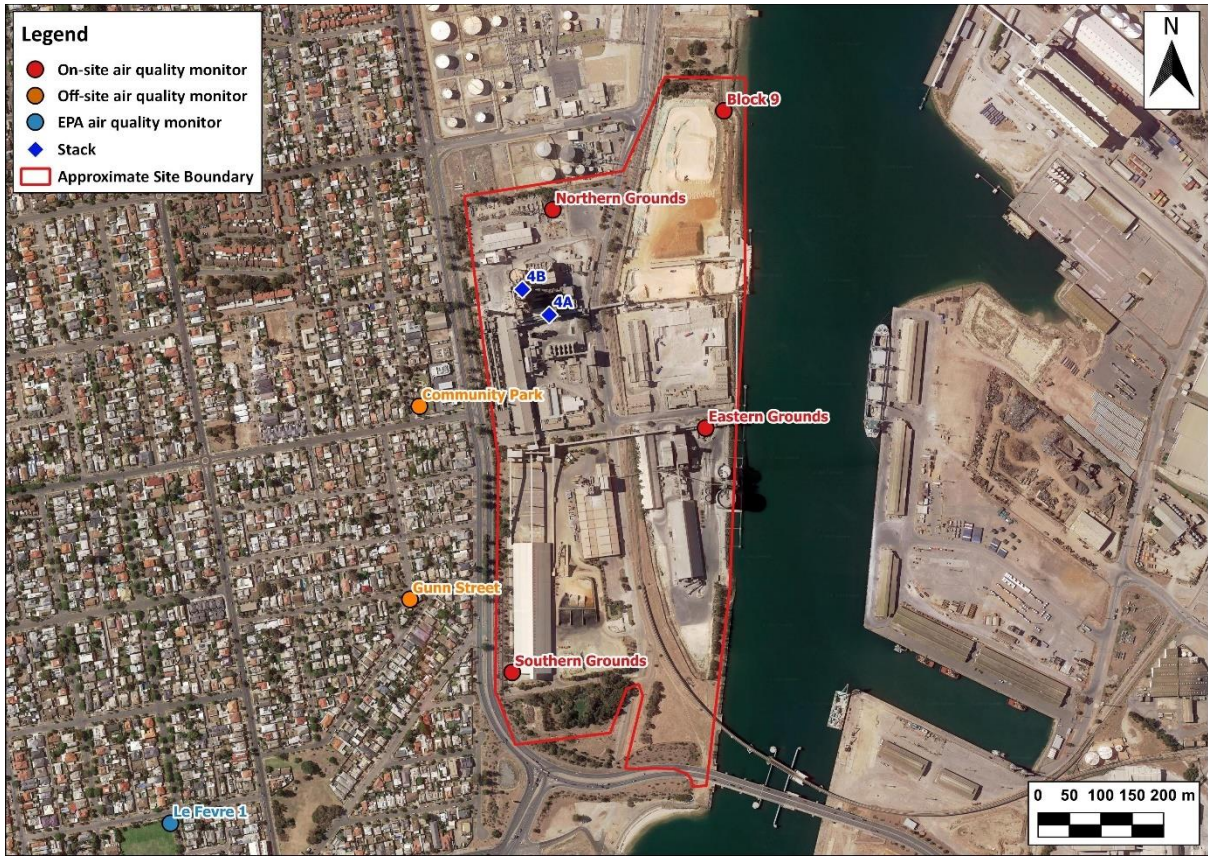
Figure 1 Site layout and ambient air quality monitors
