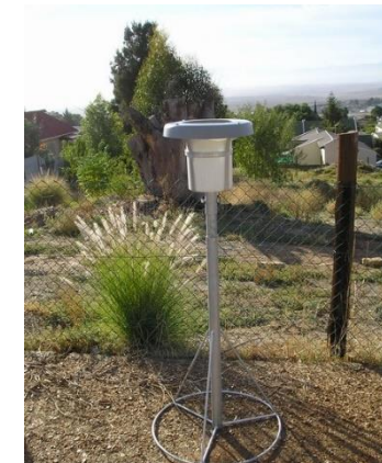
Depositional dust gauge
